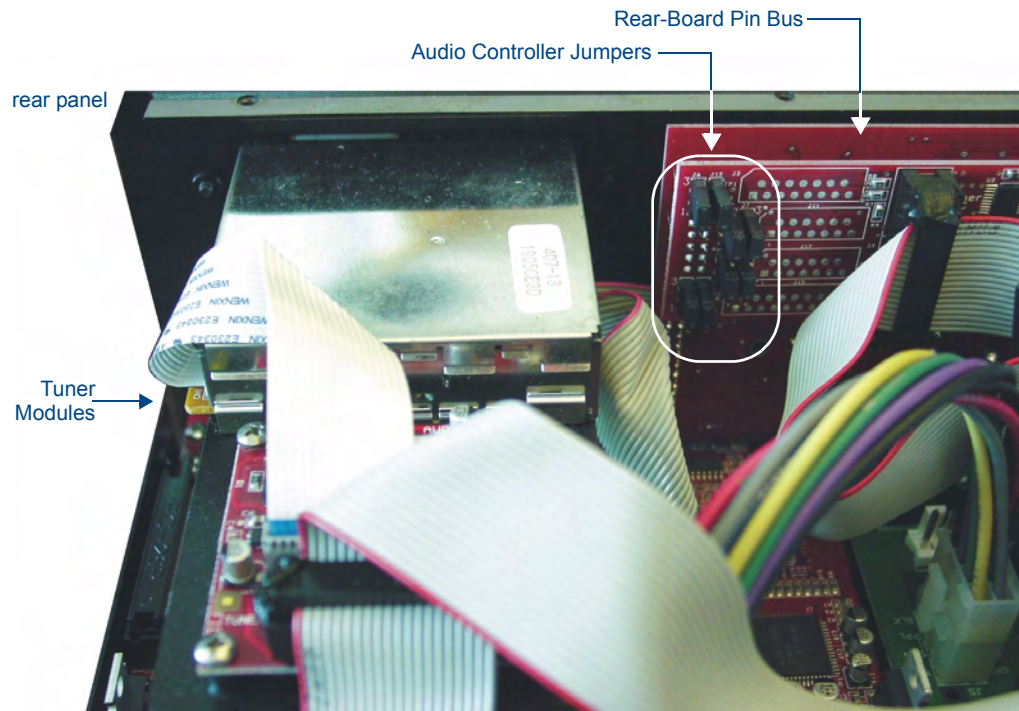
FIG. 3 Audio Controller - Rear-Board Pin Bus / Jumpers
